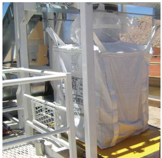
Double-lined two tonne bulk bags will be used in the sealed shipment process
